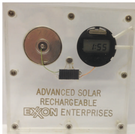
Figure 1. A LiTiS 2 cell solar rechargeable clock, built in the mid 1970s, operating in 2013.
