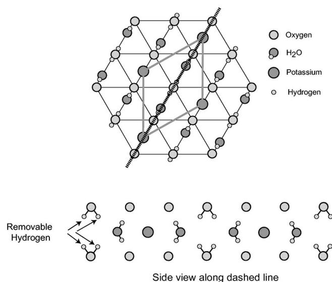
**Figure 5.** Intercalation layer of proposed crystal structure for  $\gamma$ -NiOOH. The proposed structure for  $\gamma$ -NiOOH has a P3 oxygen stacking sequence with Ni residing in octahedral sites.
