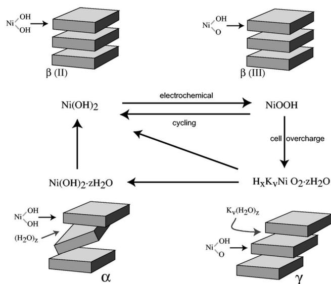
**Figure 1.** The Bode diagram illustrating the different variants of Ni-hydroxide and the possible phase transformations between them.
