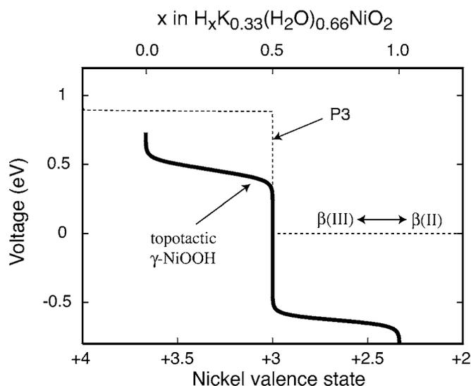
**Figure 6.** Calculated topotactic voltage curve of  $\gamma$ -NiOOH within the GGA approximation. The reference state for the anode is the same as that used in Fig. 4.
