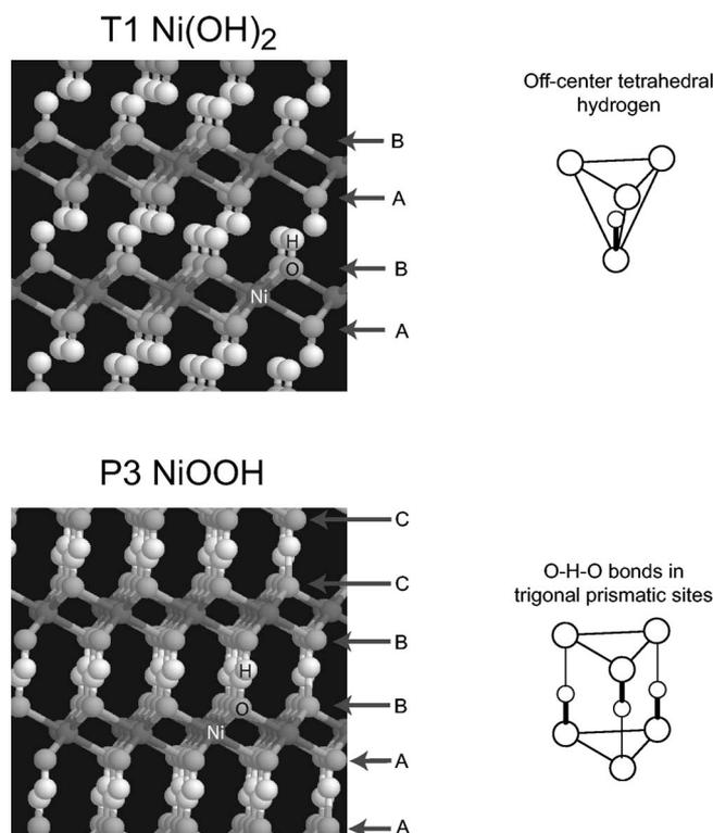
**Figure 2.** The crystal structures of  $\beta\text{-Ni}(\text{OH})_2$  having the T1 oxygen stacking sequence (ABAB) and  $\beta\text{-NiOOH}$  having the P3 oxygen stacking sequence (AAB-BCC). Also shown (right) is local coordination of hydrogen (small circles) by oxygen (large circles).
