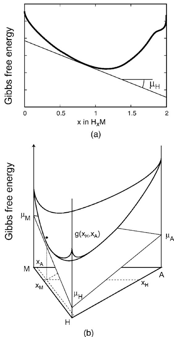
**Figure 7.** Schematic Gibbs free energies for topotactic intercalation (a) and intercalation accompanied by mass exchange with the electrolyte (b). M corresponds to the host, H to hydrogen, and A to a species of the electrolyte that can be incorporated within the host during charge and discharge.
