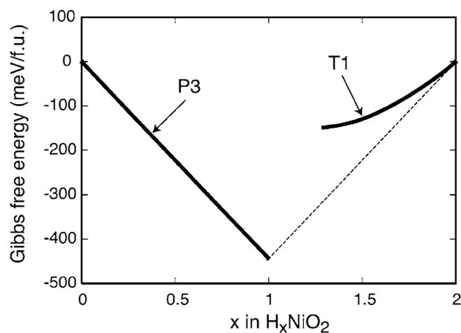
**Figure 3.** Calculated Gibbs free energies for the T1 and P3 forms of  $\text{H}_x\text{NiO}_2$ . The dashed line corresponds to the common between the T1 and P3 free energy curves and signifies a two-phase coexistence region between  $\text{Ni}(\text{OH})_2$  and  $\text{NiOOH}$ .
