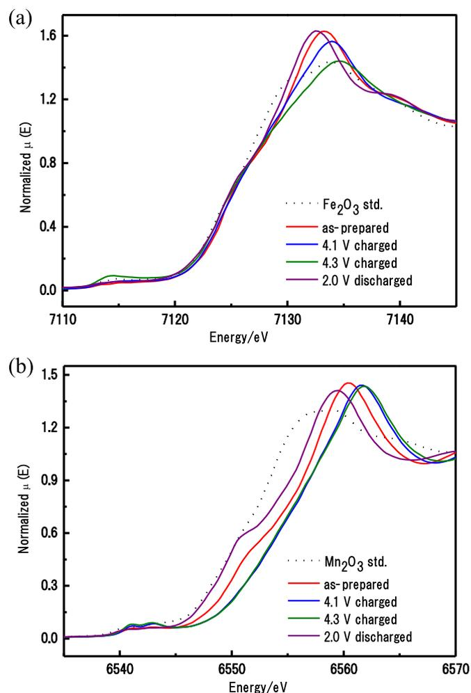
**Fig. 3.** (a) Fe K-edge and (b) Mn K-edge XAS analysis of  $\text{Na}_{2/3}\text{Fe}_{1/3}\text{Mn}_{2/3}\text{O}_2$  charged to 4.3 V and discharged to 2.0 V.
