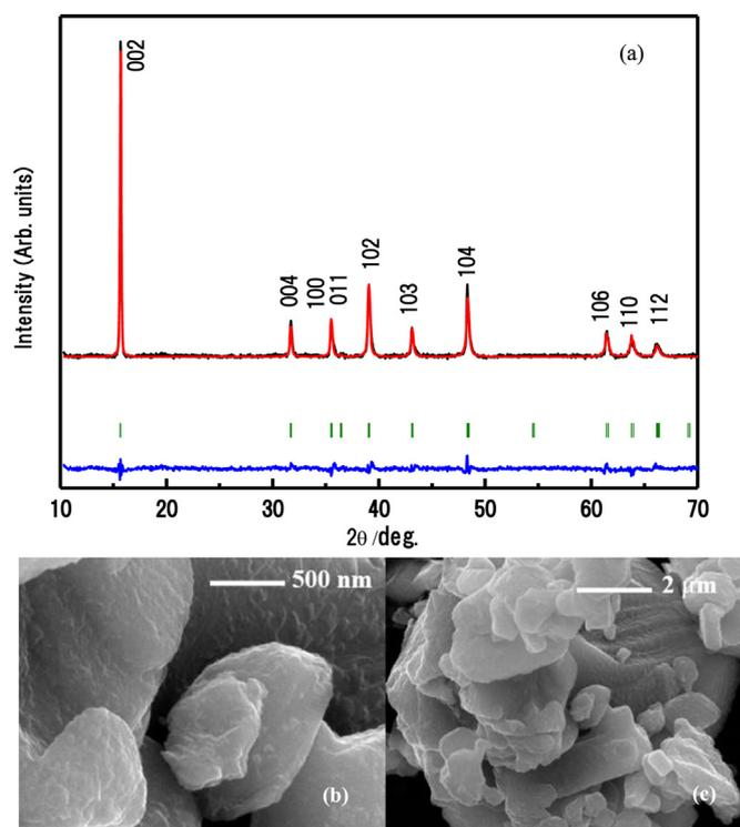
Fig. 1. (a) XRD pattern of P2-type  $\text{Na}_{2/3}\text{Fe}_{1/3}\text{Mn}_{2/3}\text{O}_2$ . The structure refinement was carried out by the Rietveld method using the FullProf software package. Particle morphology was observed by SEM at different magnifications, (b) 50000 $\times$  and (c) 12500 $\times$ .
