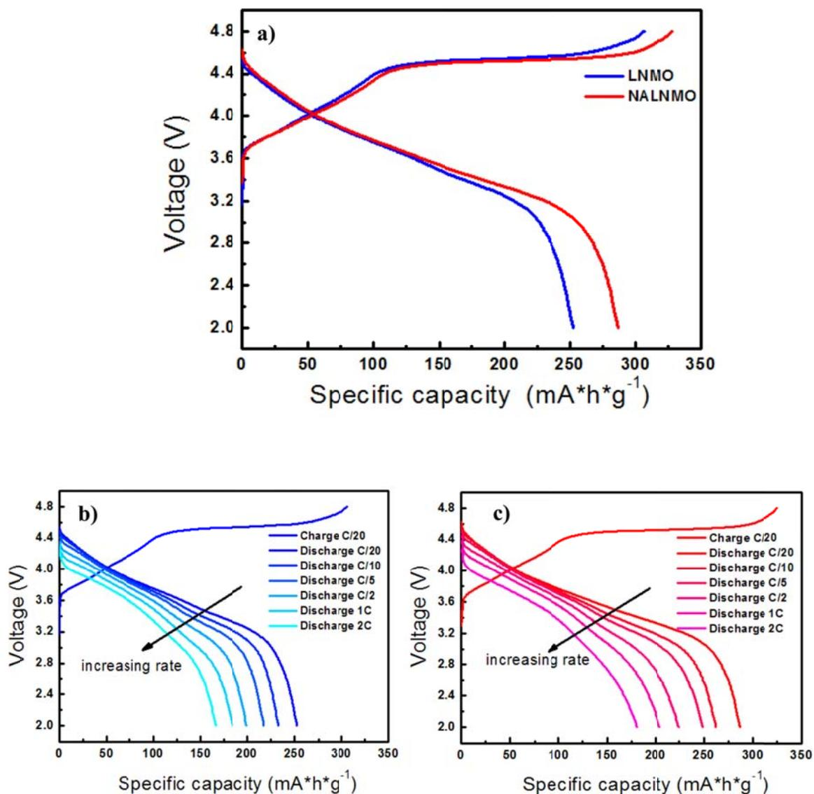
Figure 5.4 Comparison of electrochemical performances between LNMO and NALNMO. (a) first cycle charge/ discharge voltage profile, (b) voltage profile of LNMO under different current density, (c) voltage profile of NALNMO under different current density. Voltage range is 2.0 - 4.8 V at  $1\text{C} = 250\text{ mA g}^{-1}$ .
