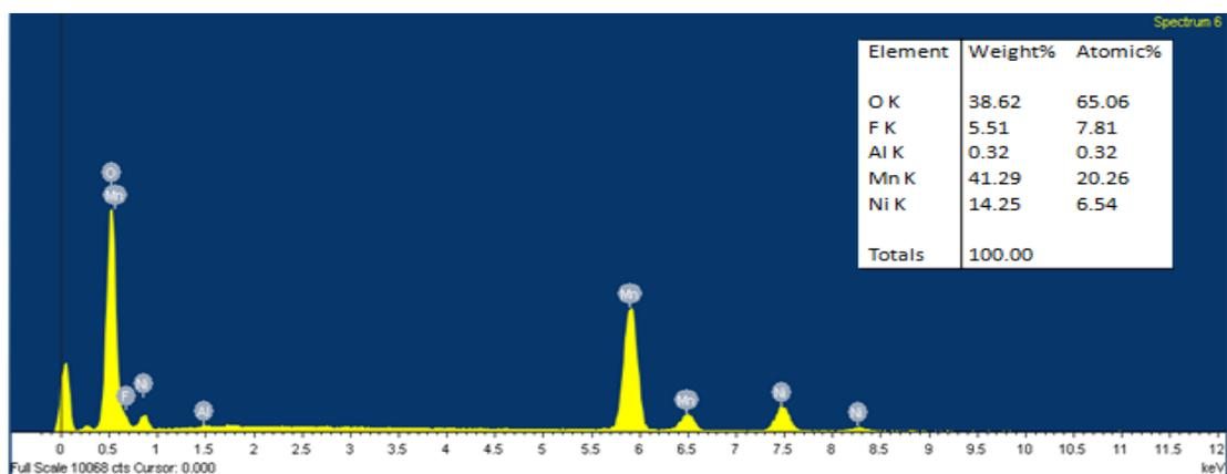
Figure 5.2 EDS spectrum of NALNMO starting material.
