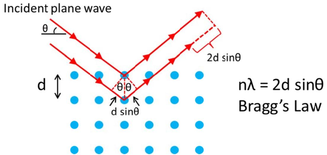
Figure 2.1 Two dimensional illustration of Bragg's law.
