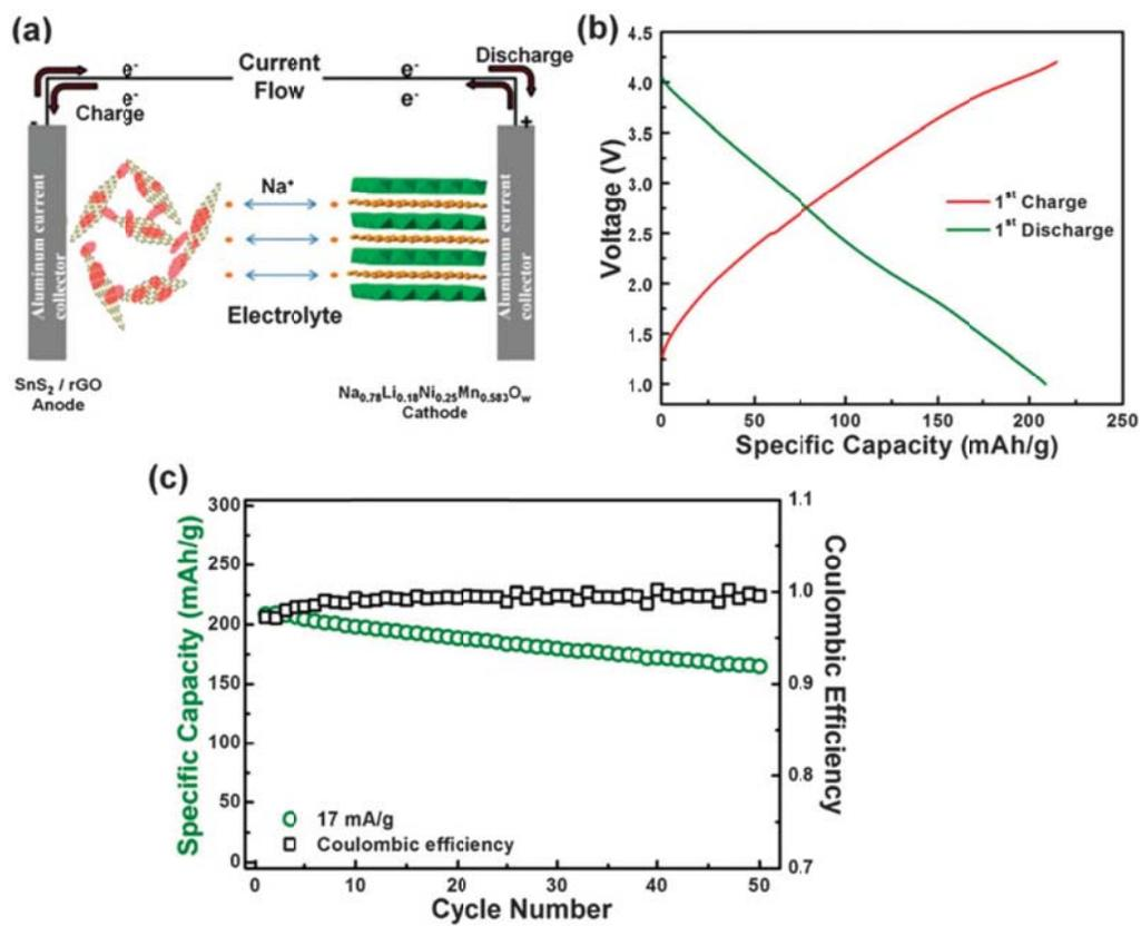
Figure 7.7 (a) Schematic of Na full cell. (b) The electrochemical profile at 1<sup>st</sup> cycle and (c) cycling performance for the Na full cell.
