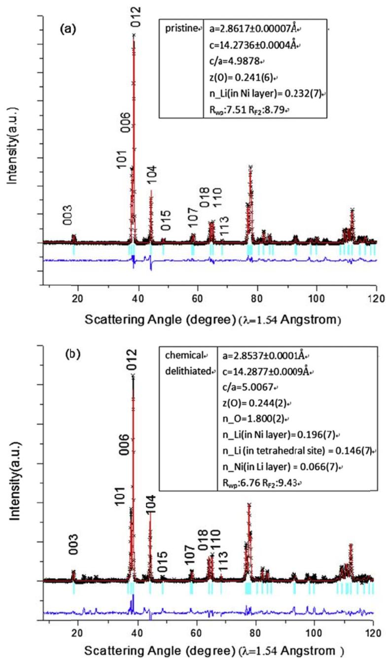
Figure 3.5 *Ex-situ* Neutron Diffraction patterns and Rietveld Refinement results: (a) pristine  $\text{Li}[\text{Li}_{0.2}\text{Ni}_{0.2}\text{Mn}_{0.6}]\text{O}_2$ ; (b) chemically delithiated sample  $\text{Li}_{0.4}\text{Ni}_{0.2}\text{Mn}_{0.6}\text{O}_{1.8}$ .
