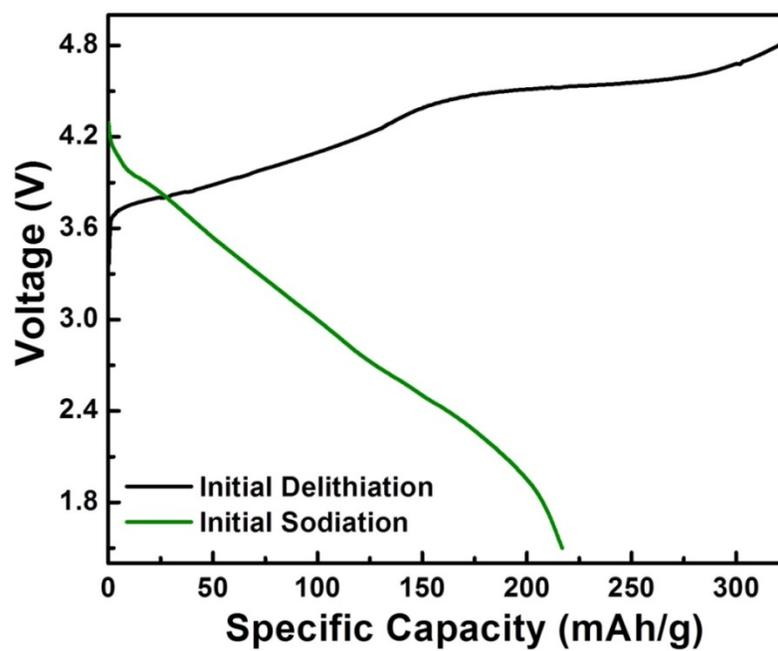
Figure 7.1 Electrochemical profile for  $\text{Li}_{1.133}\text{Ni}_{0.3}\text{Mn}_{0.567}\text{O}_2$  during initial delithiation and initial sodiation.
