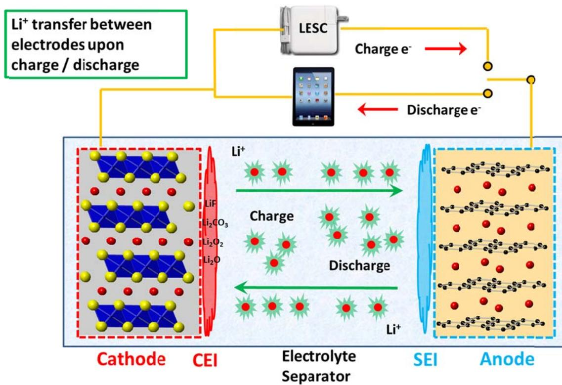
Figure 1.1 Schematic of a rechargeable Li-ion battery.
