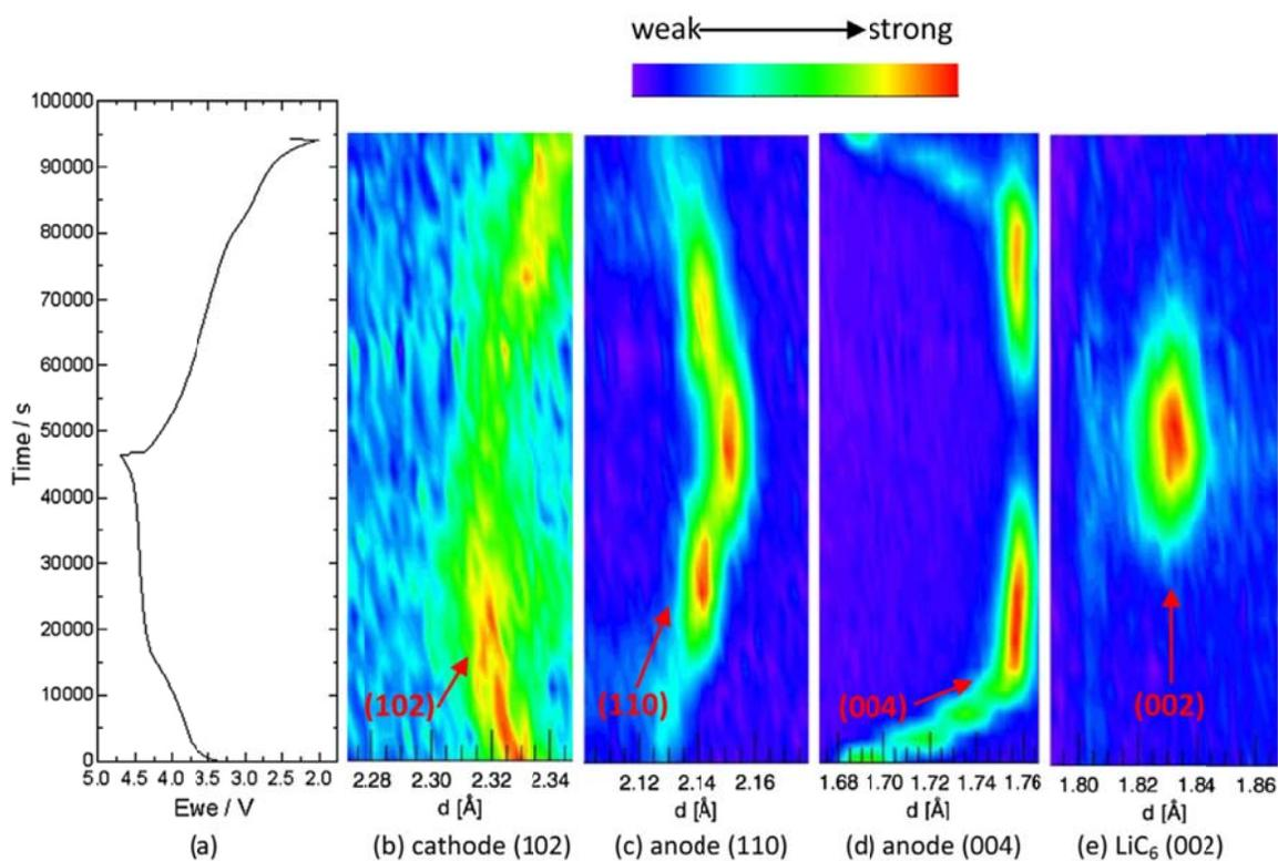
Figure 3.3 (a) 1<sup>st</sup> cycle charge/discharge curve of  $\text{Li}[\text{Li}_{0.2}\text{Ni}_{0.18}\text{Mn}_{0.53}\text{Co}_{0.1}]\text{O}_2$  and surface contour plots of (b)  $\text{Li}[\text{Li}_{0.2}\text{Ni}_{0.18}\text{Mn}_{0.53}\text{Co}_{0.1}]\text{O}_2$  (102); (c)  $\text{Li}_x\text{C}_6$  (110); (d)  $\text{Li}_x\text{C}_6$  (004); (e)  $\text{LiC}_6$  (002) Neutron Diffractions.
