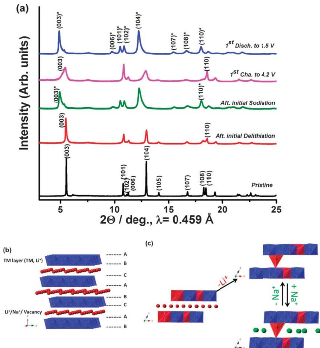
Figure 7.5 (a) Ex situ SXR D for  $\text{Li}_{1.167}\text{Ni}_{0.25}\text{Mn}_{0.583}\text{O}_2$  and  $\text{Na}_{0.78}\text{Li}_{0.18}\text{Ni}_{0.25}\text{Mn}_{0.583}\text{O}_w$  at different states. (b) Schematic of the typical O3 structure. (c) Schematic of the proposed mechanism for sodiation. (In the schematic, transition metal ions are blue,  $\text{Li}^+$  is red, and  $\text{Na}^+$  is green.)
