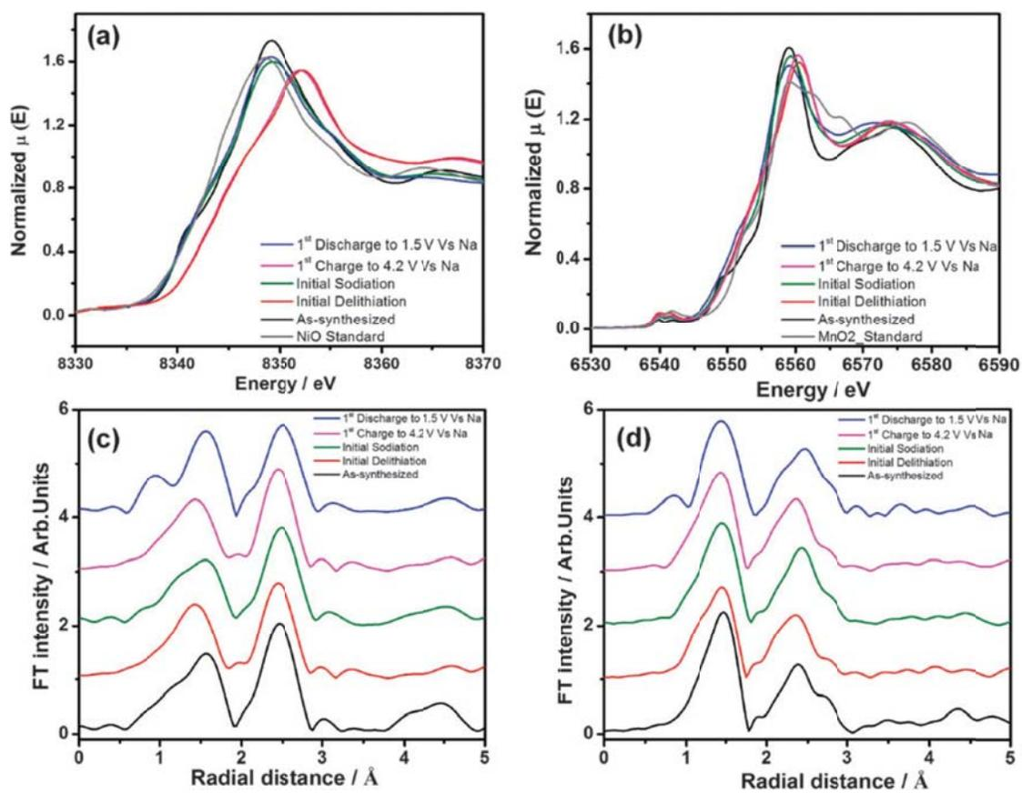
Figure 7.6 XAS analysis for  $\text{Li}_{1.167}\text{Ni}_{0.25}\text{Mn}_{0.583}\text{O}_2$  and  $\text{Na}_{0.78}\text{Li}_{0.18}\text{Ni}_{0.25}\text{Mn}_{0.583}\text{O}_w$  at different states. XANES spectra for (a) Ni and (b) Mn K-edge respectively. EXAFS spectra for (c) Ni and (d) Mn K-edge respectively.
