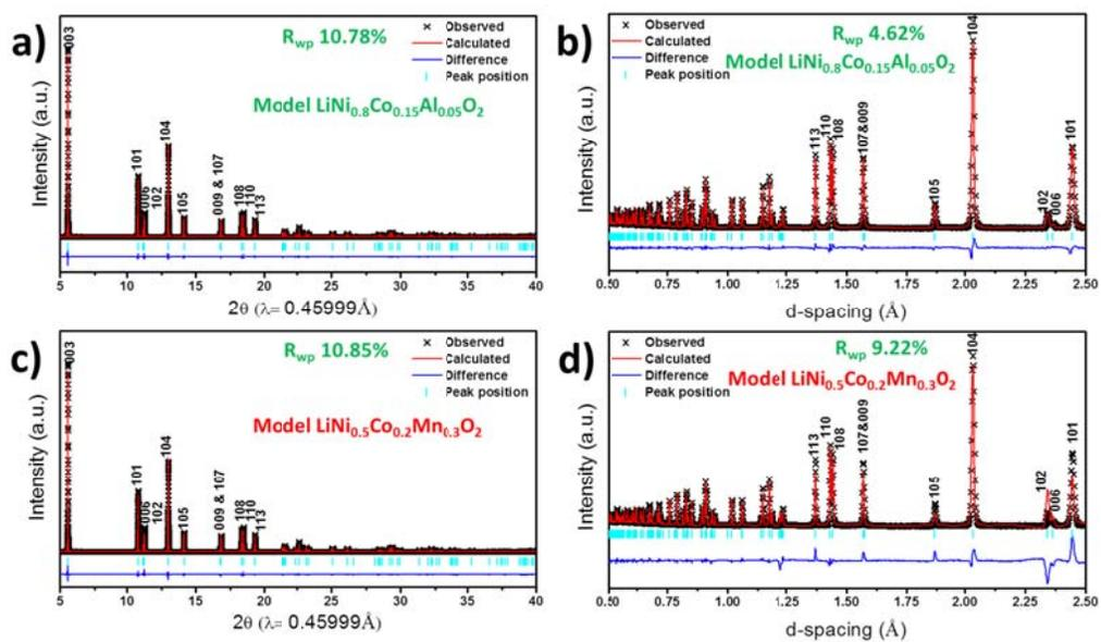
Figure 2.4 The XRD of  $\text{LiNi}_{0.8}\text{Co}_{0.15}\text{Al}_{0.05}\text{O}_2$  (a) using  $\text{LiNi}_{0.8}\text{Co}_{0.15}\text{Al}_{0.05}\text{O}_2$  model; (c) using  $\text{LiNi}_{0.5}\text{Co}_{0.2}\text{Mn}_{0.3}\text{O}_2$  model. The ND of  $\text{LiNi}_{0.8}\text{Co}_{0.15}\text{Al}_{0.05}\text{O}_2$  (b) using  $\text{LiNi}_{0.8}\text{Co}_{0.15}\text{Al}_{0.05}\text{O}_2$  model; (d) using  $\text{LiNi}_{0.5}\text{Co}_{0.2}\text{Mn}_{0.3}\text{O}_2$  model.
