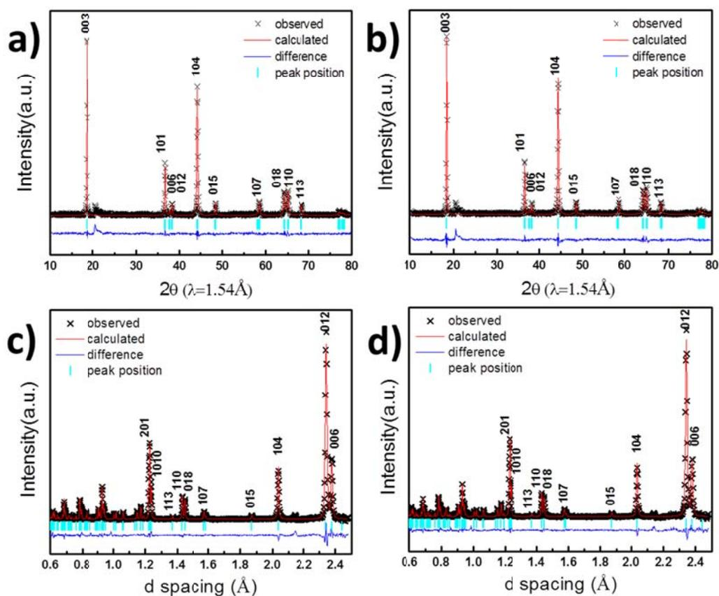
Figure 2.3 (a) The XRD of  $\text{Li}_{1.2}\text{Ni}_{0.2}\text{Mn}_{0.6}\text{O}_2$ . (b) The XRD of surface modified  $\text{Li}_{1.2}\text{Ni}_{0.2}\text{Mn}_{0.6}\text{O}_2$ . (c) The ND of  $\text{Li}_{1.2}\text{Ni}_{0.2}\text{Mn}_{0.6}\text{O}_2$ . (d) The ND of surface modified  $\text{Li}_{1.2}\text{Ni}_{0.2}\text{Mn}_{0.6}\text{O}_2$ .
