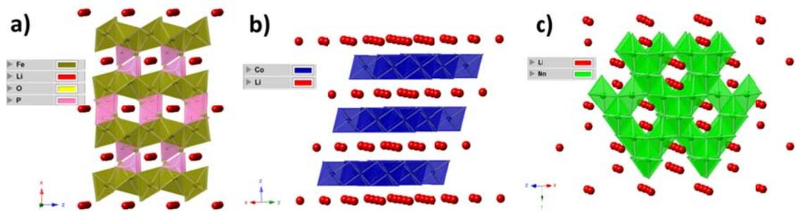
Figure 1.2 Schematics of crystal structures of a) LiFePO<sub>4</sub>, b) LiCoO<sub>2</sub>, and c) LiMn<sub>2</sub>O<sub>4</sub>.
