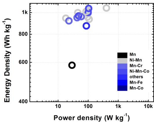
Figure 1.4 Ragone plot at the material level exhibiting the highest first discharge capacity for each year from Figure 1.3 (dashed black line).
