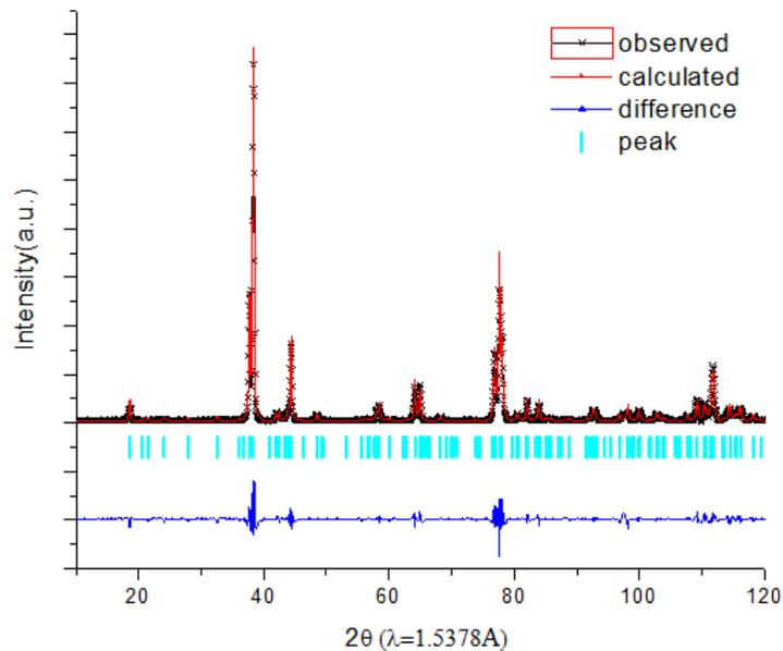
Figure 3.7 *Ex-situ* neutron diffraction patterns and profile matching with  $P3_112$  space group result of pristine  $\text{Li}[\text{Li}_{0.2}\text{Ni}_{0.2}\text{Mn}_{0.6}]\text{O}_2$ .
