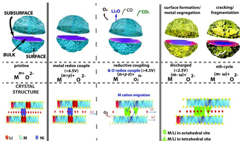
Figure 1.5 Schematic diagram of the changes that occur during electrochemical cycling that occurs within the surface and the crystal structure. The middle represents the changes in the redox for the cation and anions that participate in the charging compensation mechanism.
