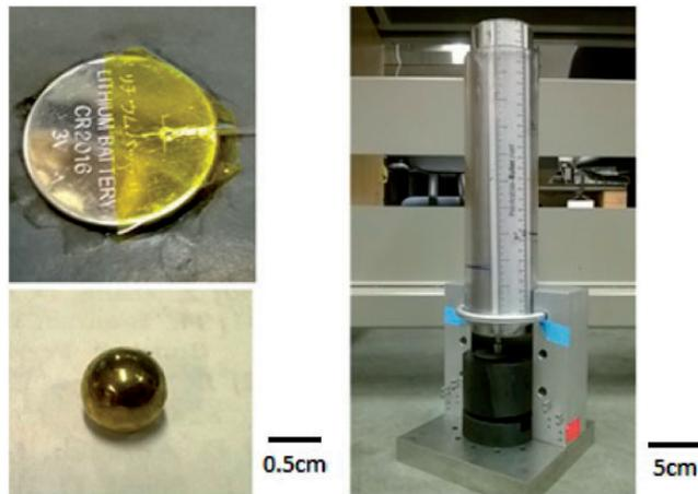
**Figure 3.** Photos of the impact experimental setup. Upper left: a CR2016 battery cell with a thermocouple attached on its upper surface; lower left: a copper spherical indenter; right: the table-top drop tower.
