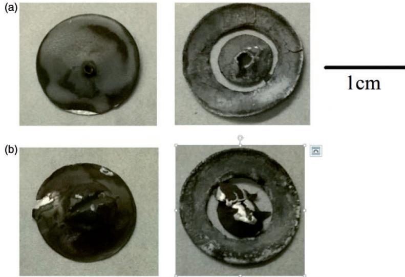
**Figure 5.** Typical reference electrode layers (left) and modified electrode layers (right) after (a) nail penetration and (b) impact tests.
