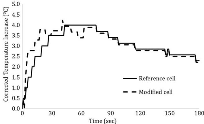
**Figure 4.** Typical temperature profiles in impact tests.
