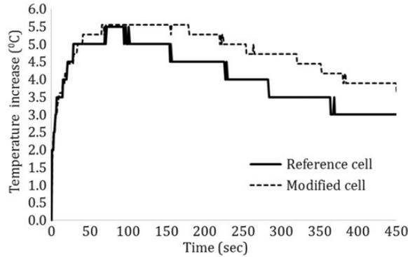
**Figure 2.** Typical temperature profiles in nail penetration tests.
