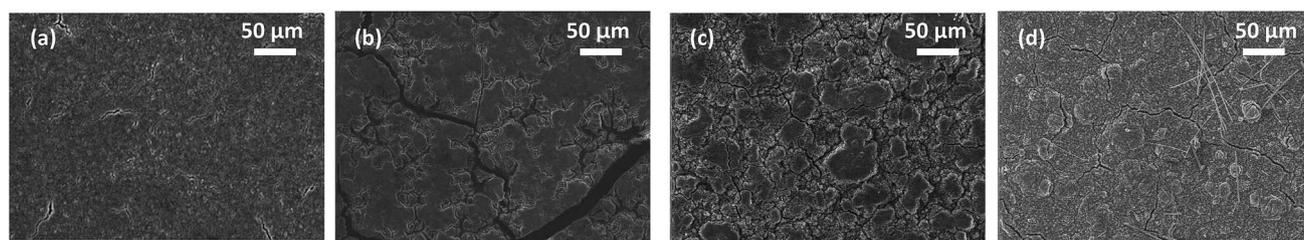
Fig. 2 SEM images of the Si anode surface (a) in its pristine state, and after 100 cycles with (b) LiPF<sub>6</sub>/EC/DEC, (c) LiPF<sub>6</sub>/EC/DEC/FEC and (d) LiFSI/EMI/FSI.
