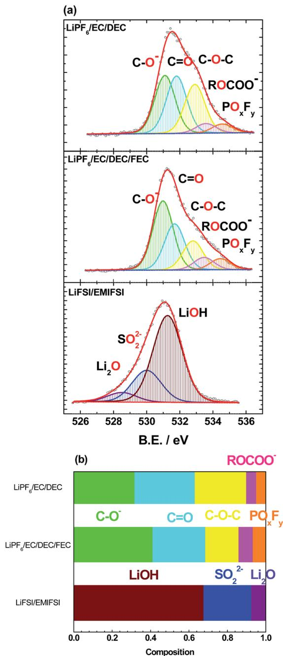
Fig. 6 (a) O 1s spectra of the Si composite anode after 100 cycles with LiPF<sub>6</sub>/EC/DEC, LiPF<sub>6</sub>/EC/DEC/FEC and LiFSI/EMIFSI. (b) Relative composition of the SEIs based on the O 1s spectra.
