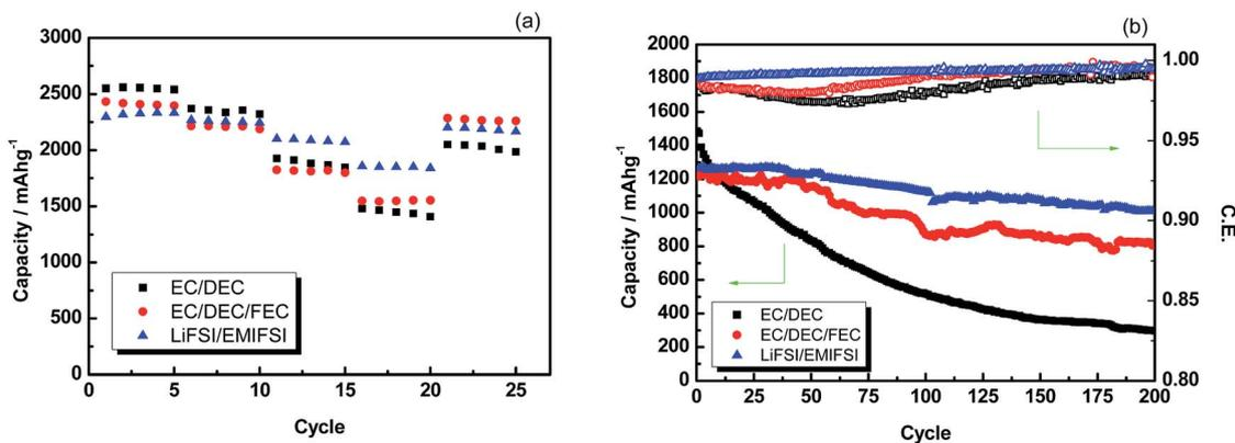
Fig. 5 (a) Rate capabilities and (b) long term 2C rate cycle performances of the Si anode with LiPF<sub>6</sub>/EC/DEC, LiPF<sub>6</sub>/EC/DEC/FEC and LiFSI/EMIFSI. Specific capacity (closed symbols) and C.E. (open symbols).
