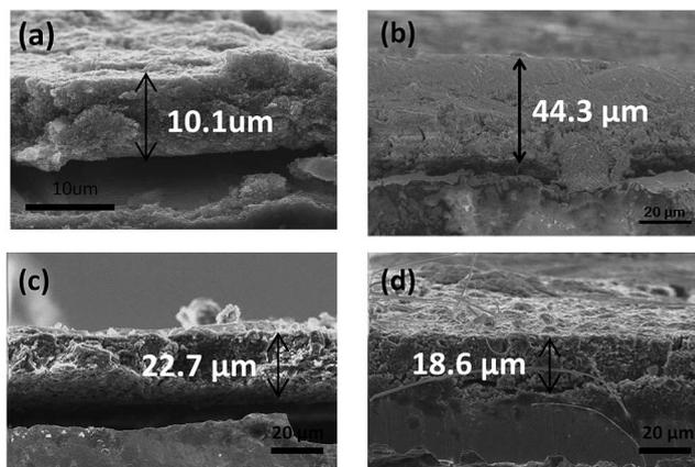
Fig. 3 Cross-sectional SEM images of the Si composite anode (a) in its pristine state, and after 100 cycles with (b) LiPF<sub>6</sub>/EC/DEC, (c) LiPF<sub>6</sub>/EC/DEC/FEC and (d) LiFSI/EMIFSI.
