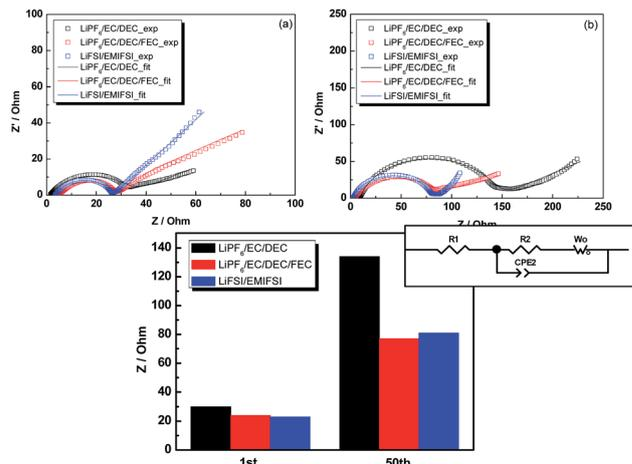
Fig. 4 EIS spectra of (a) the first and (b) the 50<sup>th</sup> cycle for LiPF<sub>6</sub>/EC/DEC, LiPF<sub>6</sub>/EC/DEC/FEC and LiFSI/EMIFSI in the lithiated state. An equivalent circuit is used to model the reaction on the Si anode. The fits for the data of each anode are shown as (c)  $R_2$  impedance between the first cycle and the 50<sup>th</sup> cycle with LiPF<sub>6</sub>/EC/DEC, LiPF<sub>6</sub>/EC/DEC/FEC and LiFSI/EMIFSI.
