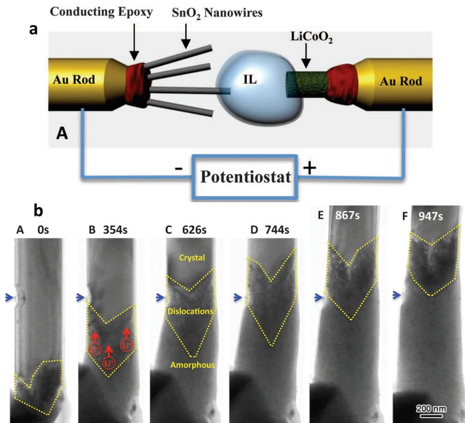
Figure 3.5: (a) Schematic of the volatile cell set up; (b) a high density of dislocations emerging from the reaction front was revealed in single SnO<sub>2</sub> nanowire.
