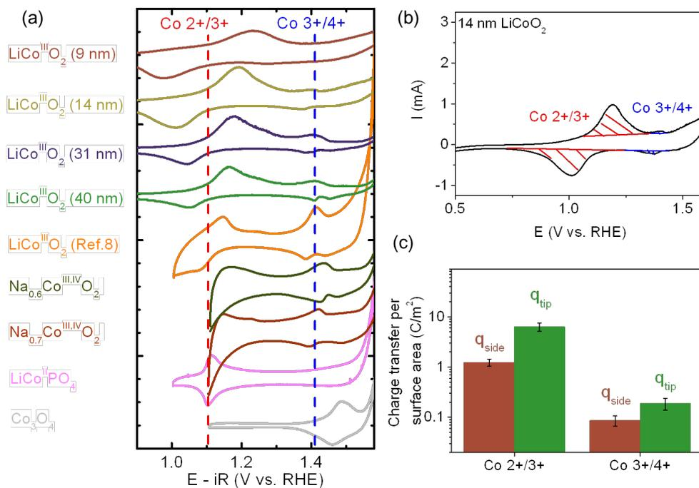
Figure 4.11: (a) CV curves of different Co compounds in the Co redox region. (b) Calculation scheme of charge transfer during Co 2+/3+ and 3+/4+ redox reactions by integrating the redox peaks. (c) Charge transferred per surface area of tip and side surfaces of  $\text{LiCoO}_2$  during 2+/3+ and 3+/4+ redox processes.
