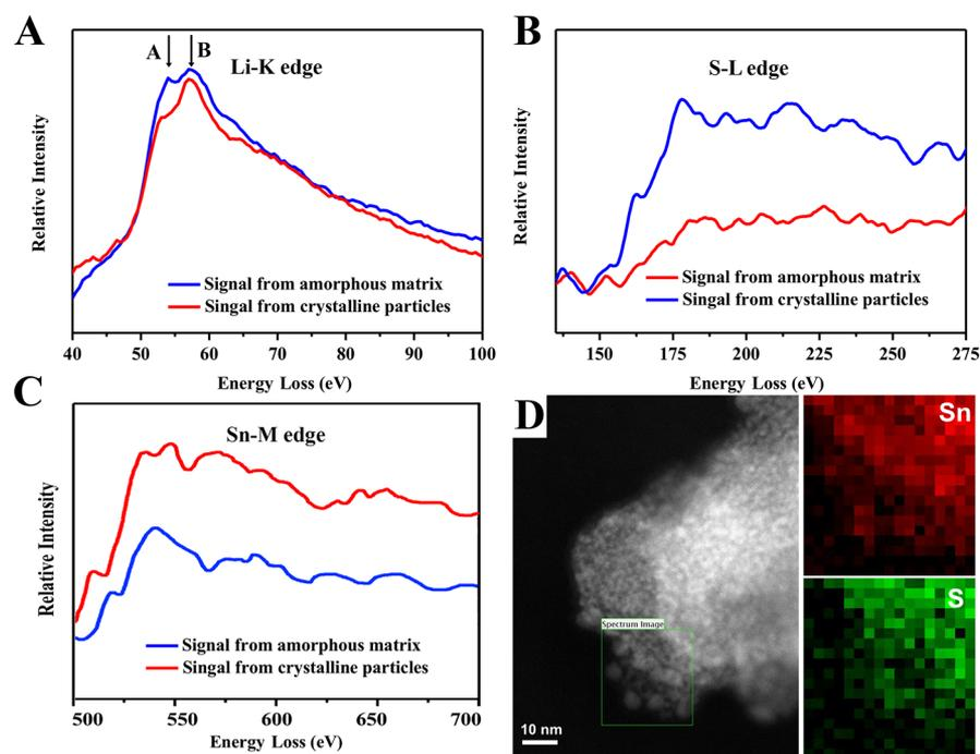
**Figure 4.** (A) Li K-edge, (B) S L-edge, and (C) Sn M-edge results for  $\text{SnS}_2$  nanocrystals lithiation reaction in different phases. (D) EELS mapping results showing that the formed particles are Sn-enriched and the amorphous phase is S-enriched.
