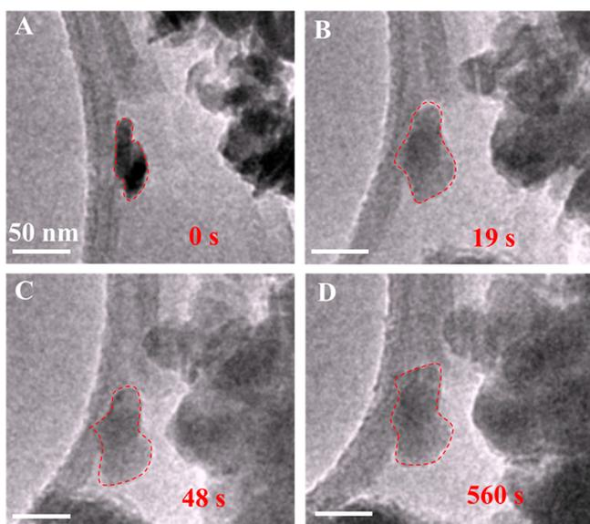
**Figure 1.** Initial lithiation process of SnS<sub>2</sub>. Time-series showing the volume expansion of SnS<sub>2</sub> nanoplates (indicated by the red dashed lines) supported on a graphene-coated lacey carbon film.
