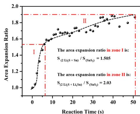
**Figure 2.** Area expansion ratio of the SnS<sub>2</sub> nanocrystals as a function of reaction time. Two different reaction speeds can be obtained. The black dashed curve shows the average trend of changes in the area expansion ratio.
