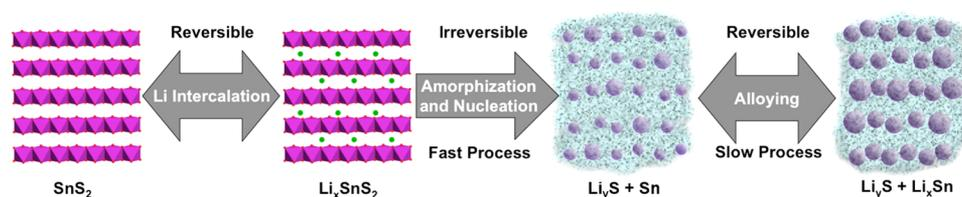
**Figure 5.** Schematic representation of the lithiation reaction for  $\text{SnS}_2$  nanocrystals. Pink, Sn; red, S; green, Li; blue matrix,  $\text{Li}_y\text{S}$ ; purple,  $\text{Li}_x\text{Sn}$ .
