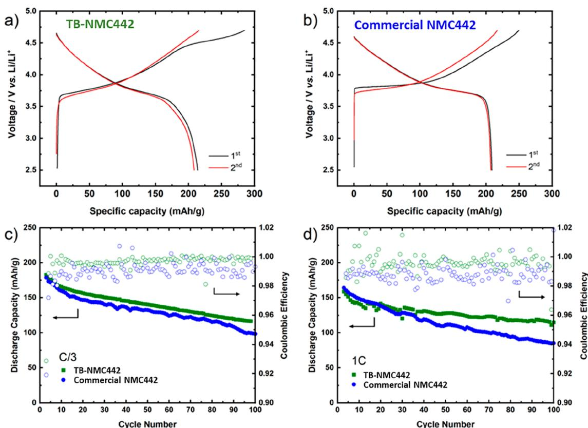
**Figure 3.** Electrochemical performance of TB-NMC442 and commercial NMC442. (a,b) Respective voltage profile of the first and second cycle and (c,d) respective cycling performance in the voltage range of 2.5–4.7 V.
