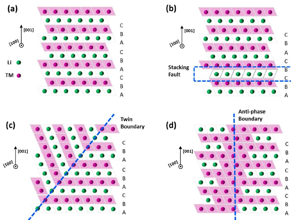
**Figure 1.** Side-view schematics of layered oxide crystals without defects and with different types of defects. (a) No defects; (b) stacking fault defect; (c) twin boundary defect; (d) antiphase boundary defect. Li ions are green circles, and TM ions are purple circles.  $\text{LiO}_6$  and  $\text{TMO}_6$  octahedra are depicted as parallelograms with Li or TM in the center.
