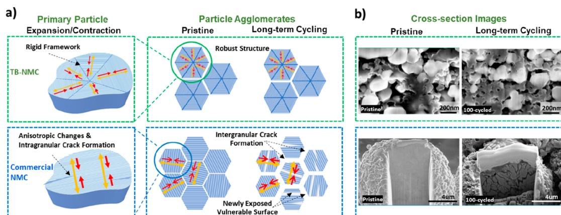
**Figure 5.** (a) Schematic of the proposed mechanism showing how TBs can alleviate  $c$ -lattice changes during cycling and mitigate intragranular and intergranular crack formation in NMC materials. (b) Cross sectional images of pristine and 100-cycled TB-NMC442 (green frames) and commercial NMC442 (blue frames).
