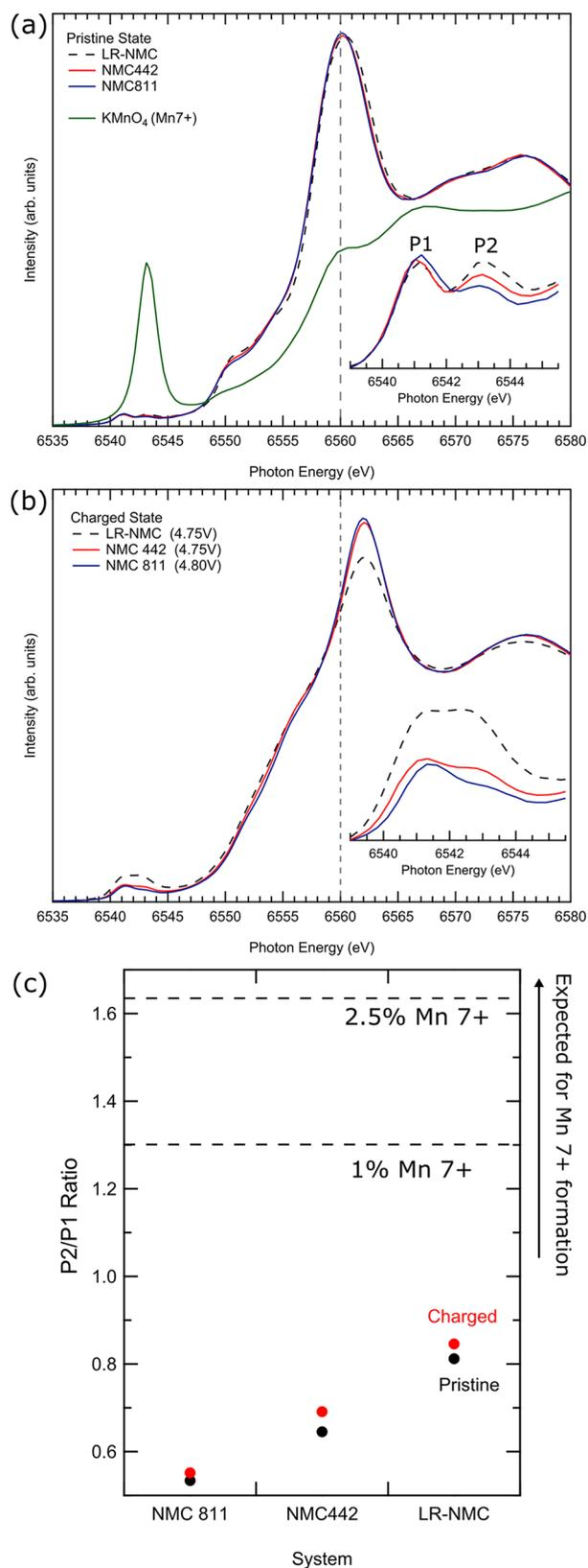
**Figure 3.** Mn K-edge spectra of (a) pristine and (b) charged states of LR-NMC, NMC 442, and NMC 811. The spectrum of  $\text{KMnO}_4$  is also plotted, which exhibits a large pre-edge feature. (c) Pre-edge P1( $t_{2g}$ ) and P2( $e_g$ ) peak intensity ratios are plotted. Horizontal lines indicated predicted peak ratio for 1% and 2.5%  $\text{Mn}^{7+}$ . Information on peak ratio predictions can be found in the Supporting Information.
