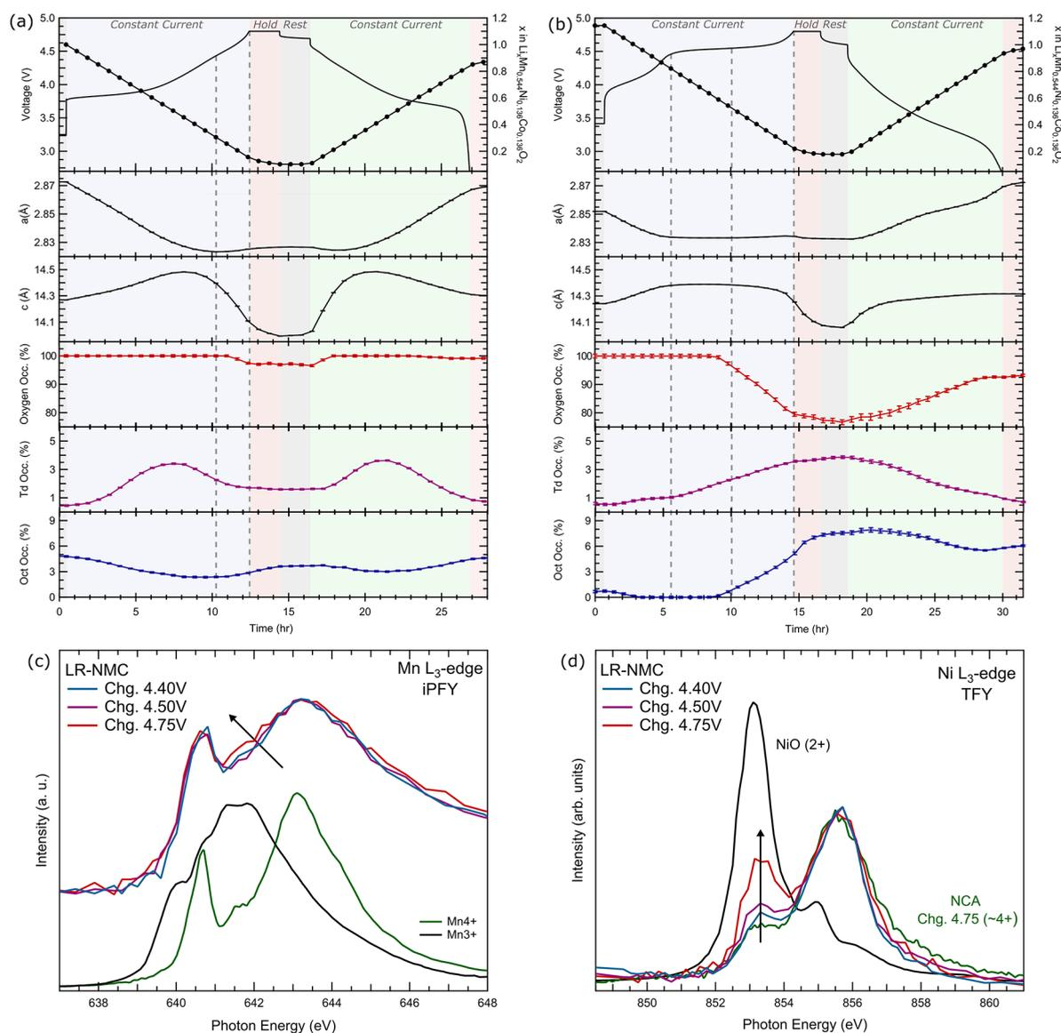
**Figure 4.** First cycle *operando* XRD data including galvanostatic charge–discharge (4.75–2.7 V) curves, *a* and *c* lattice parameters, oxygen occupancy, and TM occupancy in Li layer of (a) LR-NMC and (b) NMC 442. (c) Mn L<sub>3</sub>-edge iPFY and (d) Ni L<sub>3</sub>-edge TFY of LR-NMC electrodes with Mn and Ni reference spectra.
